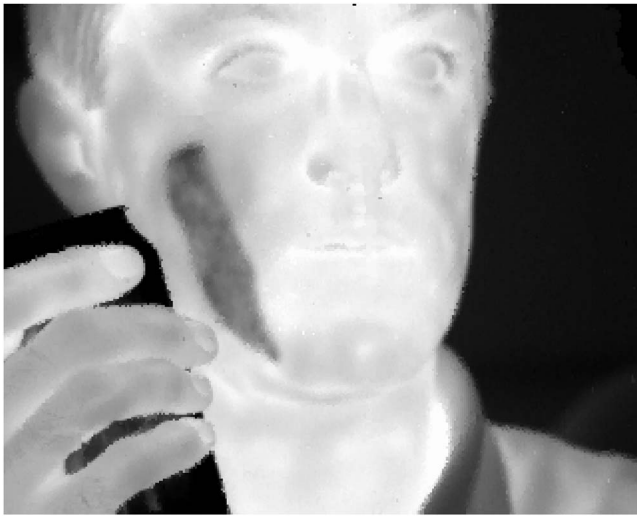
FIG. 4. Thermal image taken with 320 \times 256 InAs/GaSb SL nBn camera at a detector temperature of 77 K and integration time of 16.3 ms. Two-point NUC was utilized.
