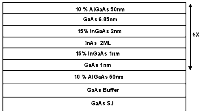
FIG. 1. Baseline structure used for optimizing the DWELL detector. The GaAs layer under the dot and the \text{In}_{0.15}\text{Ga}_{0.85}\text{As} capping layer above the dot were optimized using this structure.
