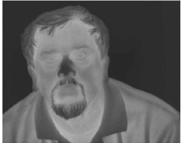
Figure 1. An image taken with the first 640 \times 512 pixel QDIP LWIR FPA operating at 60K.
